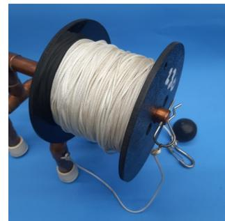
The spool has center holes in each side that are just large enough for the spool to slide on the spindle. Two additional holes are placed in each side of the spool equidistant from the center and spaced so the metal winding fork will fit into them.
