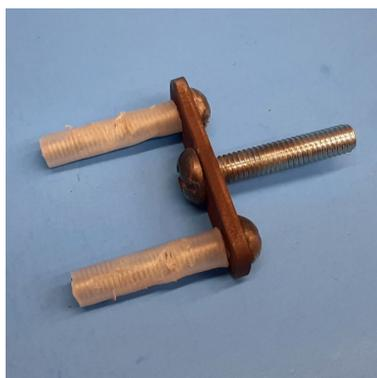
To bring the line and mark in, we use a cordless drill/driver with a winding fork made of 1/8" metal stock with three holes threaded for three machine screws that are approximately two inches long and 5/16" in diameter. Thread the screws all the way into the metal plate and stabilize them with a bit of solder or maybe Loctite will
