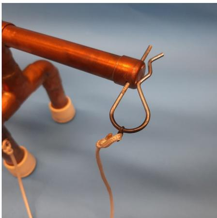
The spool holder is made of 1/2" and 3/4" copper pipe. Solder joints do not have to be water tight, only strong enough to hold the parts together. The clip goes through the hole in the cap on the end of the spool spindle to keep the spool from sliding off as the line is unwinding as the tug is pulling it out.
